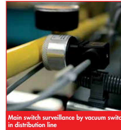
Acoustic warning unit goes off in case of vacuum decrease or power failure
