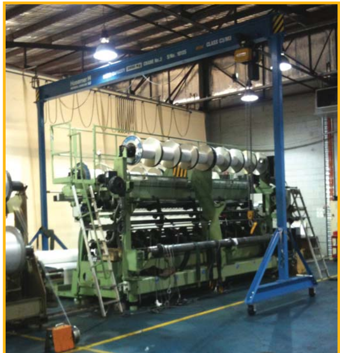
The gantry on site at Stretchtex.
